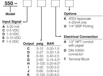
\*Output shown is as calibrated at the factory. Large span adjustment capability allows recalibration to achieve ouput ranges down to 3-35 psig (0.2-2.4 BAR) with 2-60 psig unit, and up to 3-145 psig (0.2-10.0 BAR) with 3-120 psig unit.
